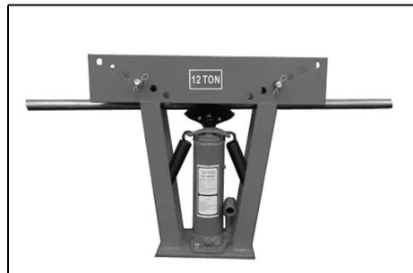
9. Continue to pump the handle and constantly monitor the bending process.
